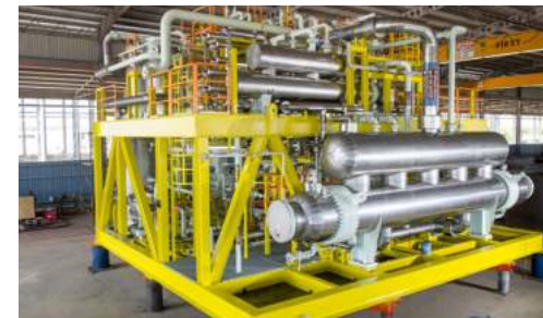
Gas de-hydration/dew point control
